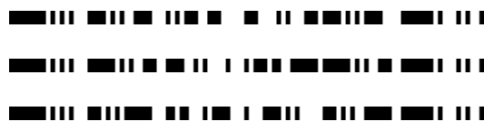
Figure 2 - Individual Rows of a PDF417 Symbol
